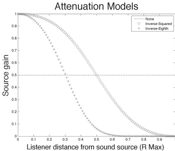
Figure 1: Attenuation Models used in each experimental condition.
